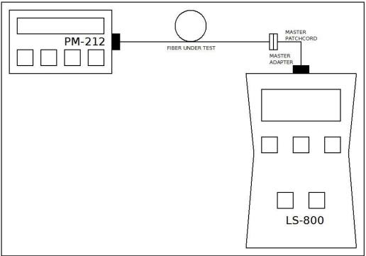
Figure 8: Mesurement Loss by method 7
