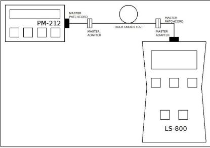
Figure 6: Measurement Loss by method 6
