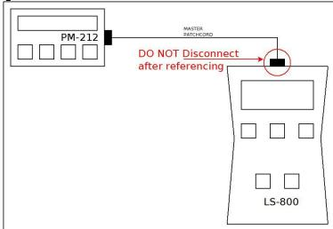
Figure 7:Setting reference by method 7
