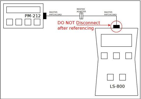
Figure 5: Setting reference by method 6
